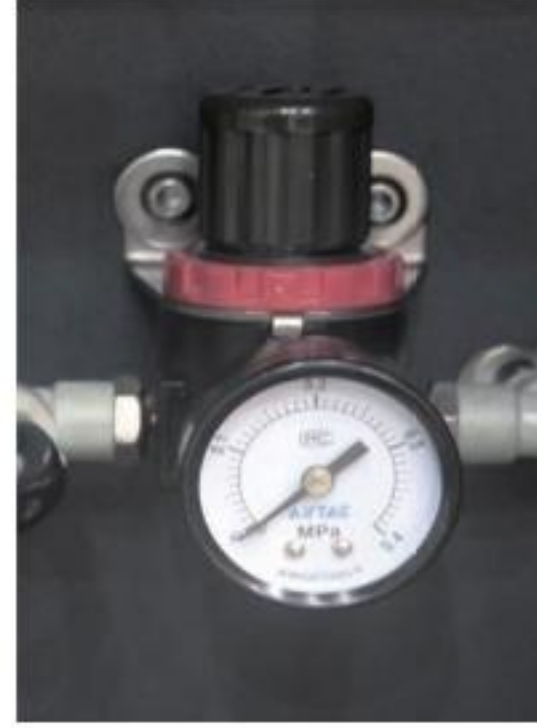
Precise pressure release valve to keep air pressure stable and extend spindle service life .
