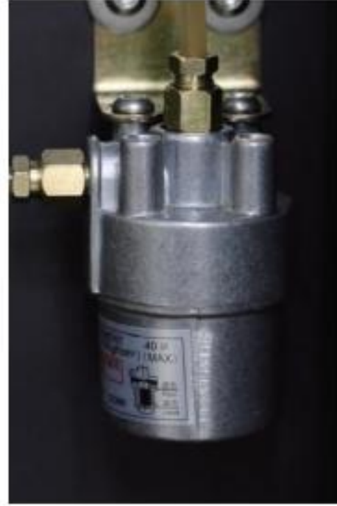
Oil filter to avoid lubrication pipeline jam .
