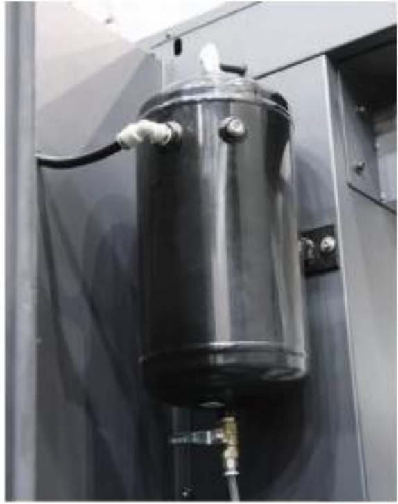
Air cylinder to effectively reduce tool changing faults .
