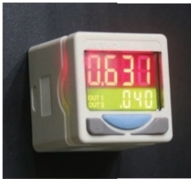
Low pressure monitor to avoid heavy damage to spindle .
