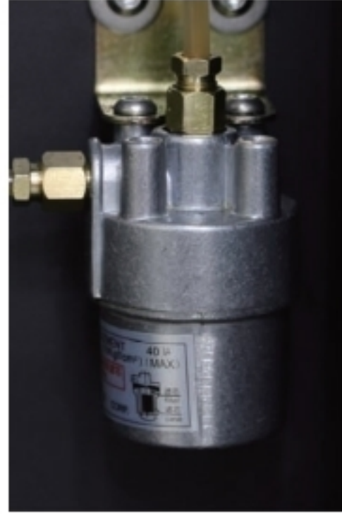
Oil filter to avoid lubrication pipeline jam .
