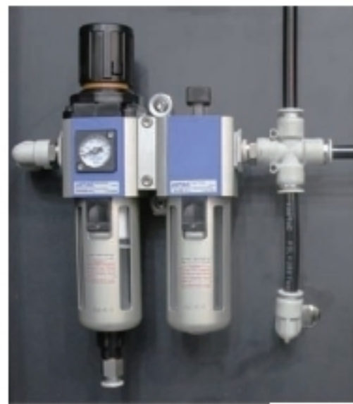
Air filter to reduce water and oil pollution in air and increase service life of spindle and ATC.
